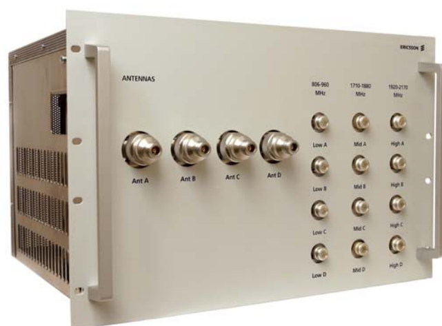
Figure 12 An example of triple band combining box. This unit can be used as the interface between a distributed antenna system and up to twelve radio base stations (up to four RBSs per band).
